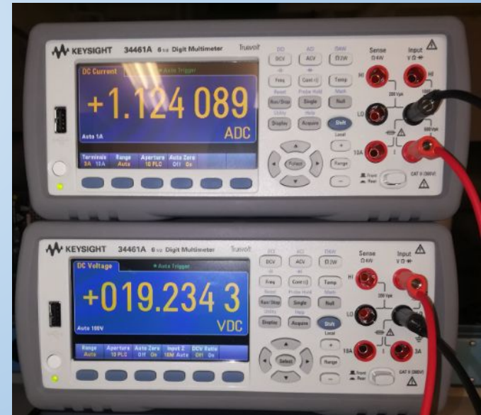
Rectified Delivered Power
